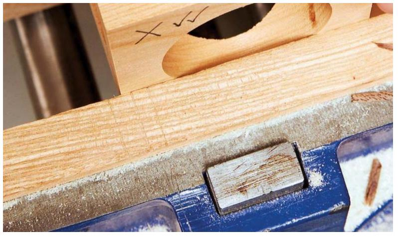
10. Release the inner cube by cutting the attachment points with a thin knife, going with the grain. After cutting all eight corners, the inner cube will drop free. But it won't come out!
