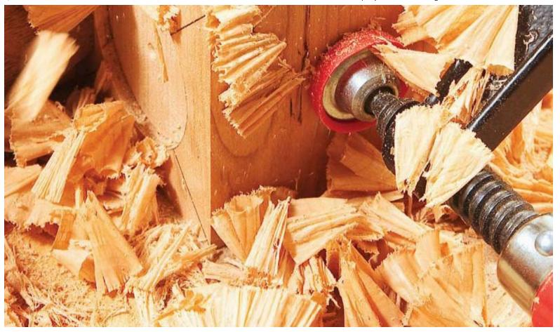
6. Drill holes in the end-grain sides first. Then drill the other four faces. Always place the X's in the same corner relative to the fence and stop block.
