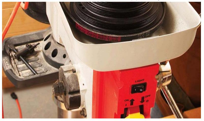
3. Set your drill press to run at its slowest speed. Arrange the belts so the smallest diameter drive pulley turns the idler pulley. Connect the idler to the largest diameter spindle pulley.
