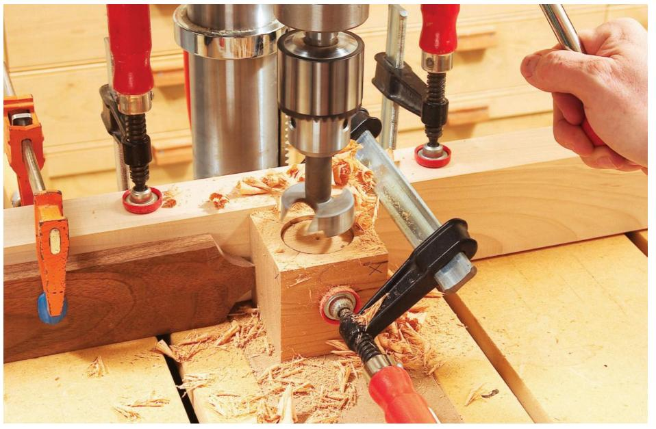
4. Set up your drill press with a 2 in. Forstner bit. (Use a smaller bit with a smaller block.) Position a fence and stop block so the bit drills exactly in the cube's center. Drill one hole about 1/16-in. deep.
