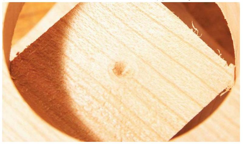
9. As you drill, check the thickness of the attachment points. Your goal is to make them as small as possible, to the point where the inner cube almost releases itself. This may require drilling some holes a tiny bit deeper. Draw check marks to show how many times you've drilled each hole.
