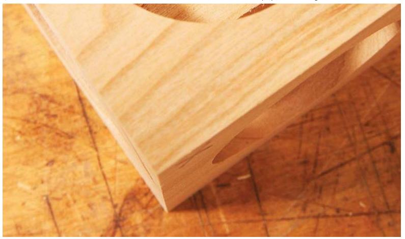
7. Drilling all six faces produces a cube in a cube. The inner cube is attached to the outer cube by a thin section of wood. The reason for drilling the end-grain faces first is to avoid breaking these weak attachment points. End-grain drilling requires more downward pressure than face-grain drilling.
