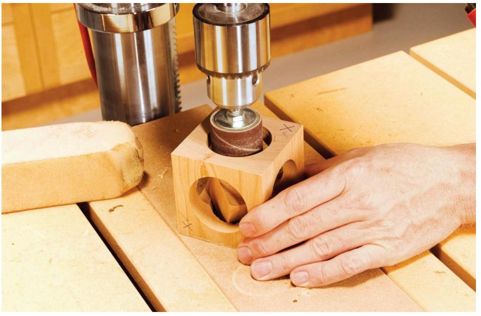
12. Sand burn marks or rough grain with a fine-grit drum-sanding attachment. Rub the drum with a crepe-rubber belt cleaner now and then to keep the drum working efficiently.
