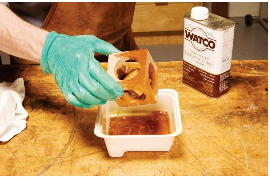
14. Dip the cube in oil to finish it. Rub thoroughly with a rag to remove the excess oil, and you're ready to play!
