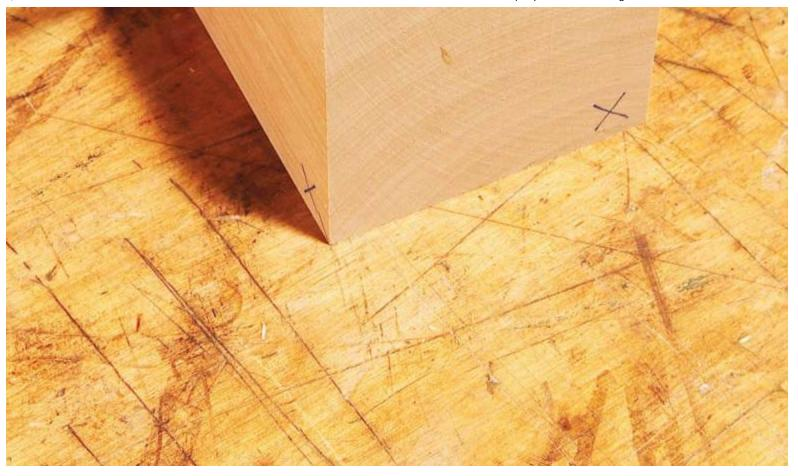
2. Mark centerlines on one face. Mark one corner of every face with a small X. You'll be drilling each hole more than one time. The X's will help register the cube in the same orientation on the drill press.
