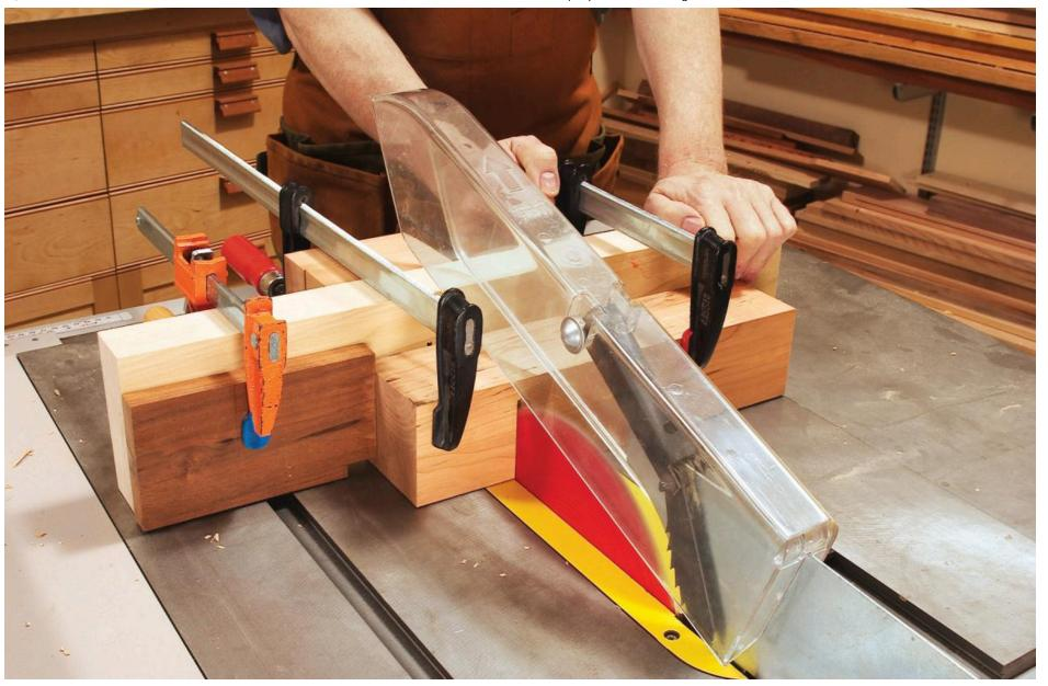
1. Crosscut a 3x3x14-in. blank into four cubes. Solid wood is best, so it doesn't look like you put the little cube in the big cube by gluing parts together. Table-leg stock works well, but you can make the cubes from smaller stock if you want.
